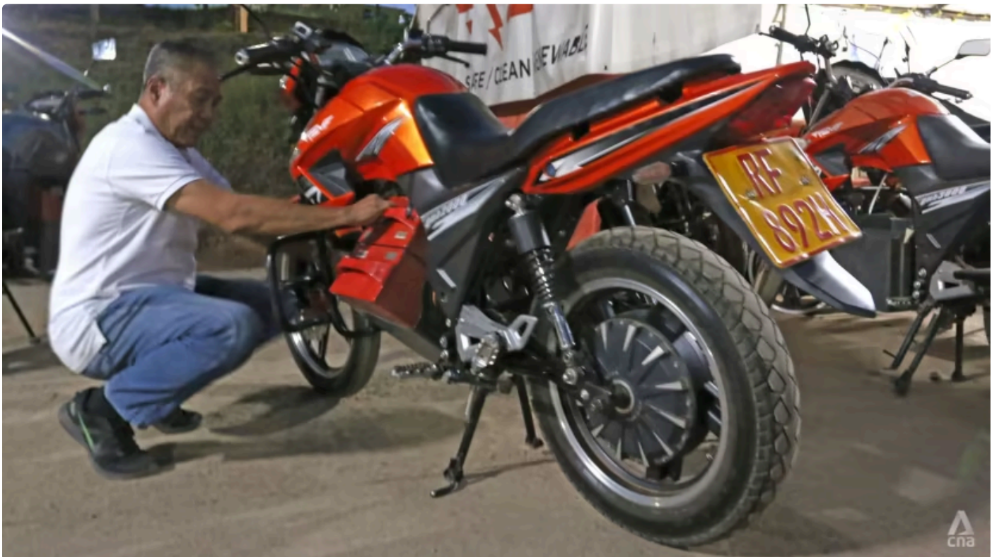
Mr Ting demonstrating how the two batteries are swapped out on REM's bike. (Photo: CNA/Aqil Haziq Mahmud)
